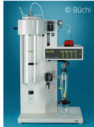
Büchi Mini Spray Dryer for laboratory scale coating experiments.
